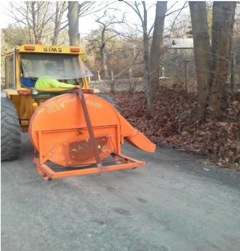
This blower that we use to blow leaves out of ditches and culvert pipes was adapted by Town of Copake Highway employees. It was originally a silage loader at a local farm.
