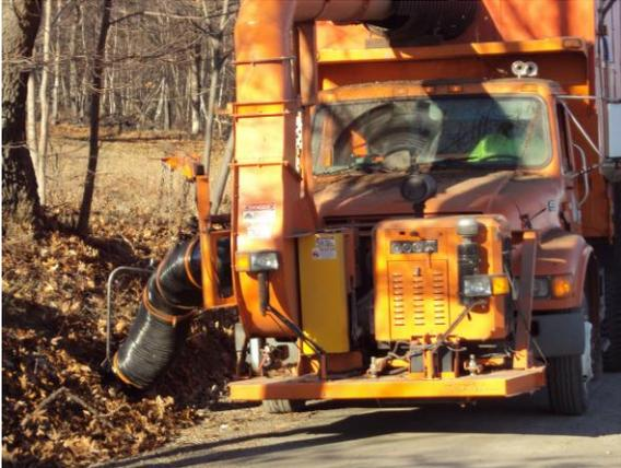
***Mounted on the front of the truck it increases efficiency by requiring only two employees. Safety is also improved as the controls are within the cab; no employees are needed outside of the truck. Working in conjunction with the truck vacuum is a tractor with a PTO driven blower. This blower was originally a silo loader. The fabrication required to modify it into a blower was also done by our employees.***
