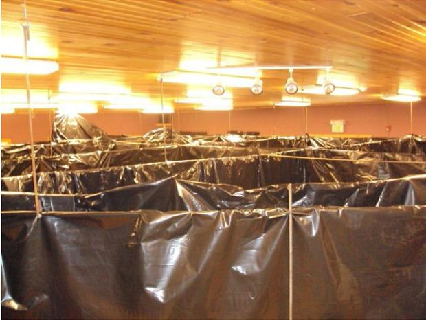
The “walls” of the haunted house are plastic sheeting hung from steel rods that are suspended from hooks in the ceiling. Each year the configuration of the rooms change requiring an adjustable system.
